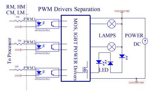
Connection should be realized as short as possible due to large currents ant short pulses of controlled signal.
