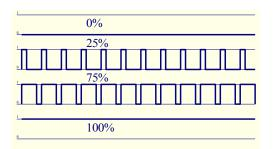
PWM outputs along to Power drivers installed optionally (with or without optoisolation for protection) on:
