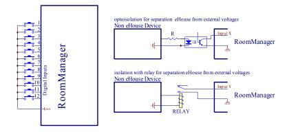
Inputs must be separated from any voltages. Only short to the ground (GND) of current controller is accepted.
