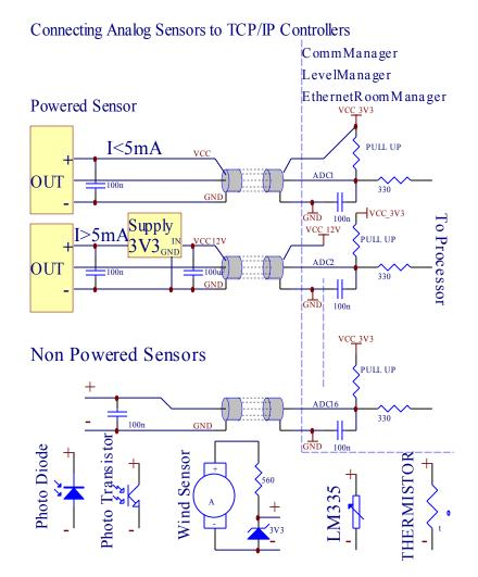
Each channel configuration of Analog to Digital Converter is realized in CommManagerCfg.exe application in "Analog to Digital Converter Settings" \* tabs.
