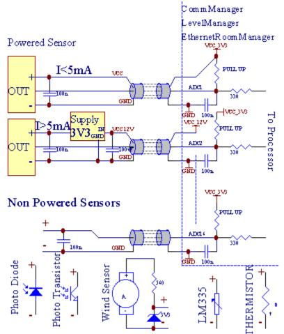
Connecting Analog Sensors to TCP/IP Controllers
