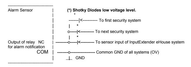
Sabotage outputs should be connected to only one system without any changes Using Diodes for separation of multiple security systems causes decreasing margin of errors and InputExtender can generate fake alarm in case of very strong disturbance (thunderbolt, close location to GSM antennas high power signals).
