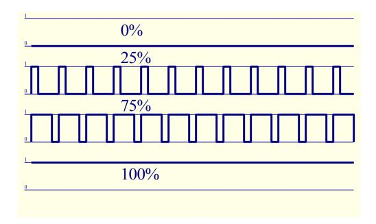
PWM outputs along to Power drivers installed optionally on Relay Module, can regulate fluently (255 positions) light level of lamps powered 12V/DC - 30W. Eventually external power drivers with opto-isolator on input, can be used to drive high power and inductive loads (e.g. DC motors, ventilators, pumps).
