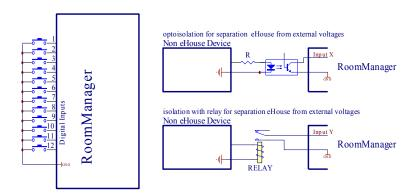
Inputs must be separated from any voltages. Only short to the ground (GND) of current controller is accepted.
