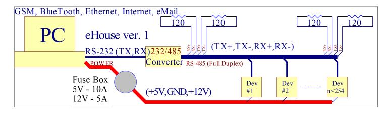
As many as 254 eHouse 1 devices can be connected to eHouse 1 bus. Devices must have unique address. Each device has 2 byte address for identification (ADRH, ADRL). Each device is pre-programed with default address (55,55). Devices must be connected to the bus one by one, and address should be changed from default, immediately after connection to unique value.
