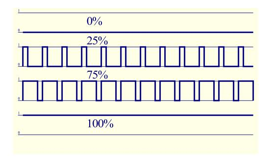
PWM outputs along to Power drivers installed optionally on Relay Module, can regulate fluently (255 positions) light level of lamps powered 12V/DC - 30W. Eventually external power drivers with opto-isolator on input, can be used to drive high power and inductive loads (e.g. DC motors, ventilators, pumps).
