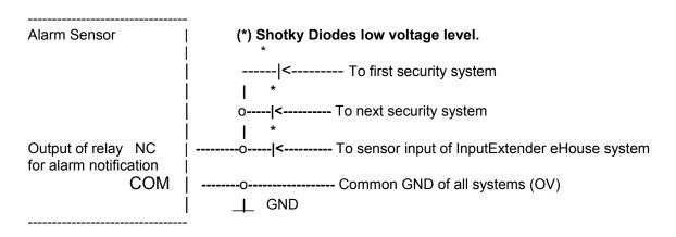
Sabotage outputs should be connected to only one system without any changes
